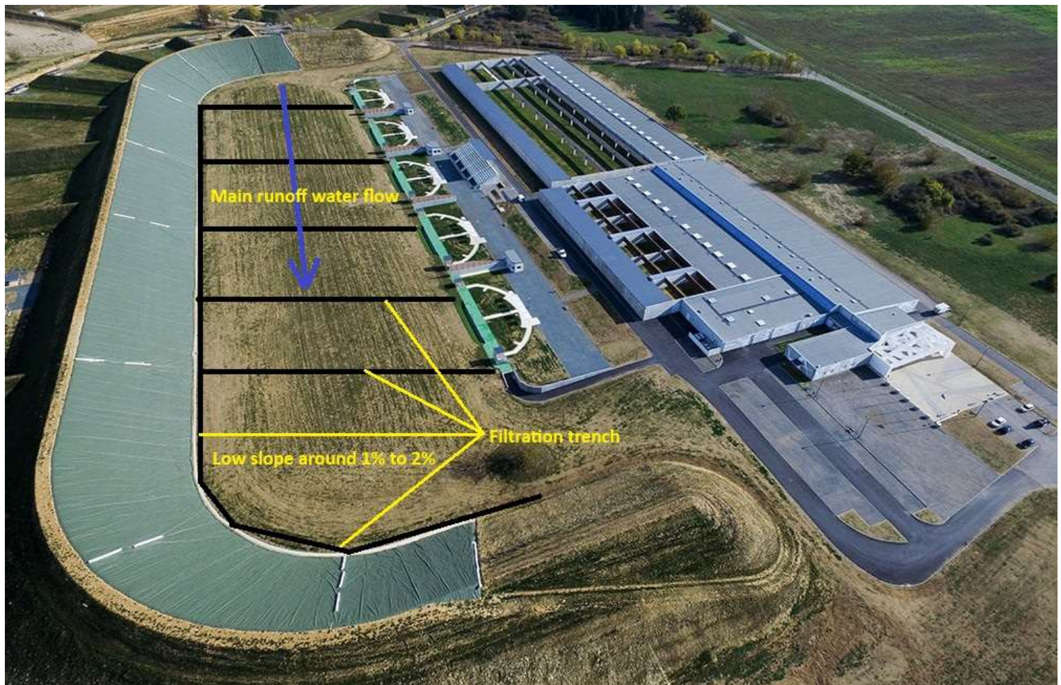
Figure 6 : conceptual design of runoff water filtration for shooting range with low slop
